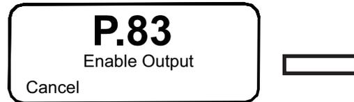
5. Turn on the power source to provide the maximum calibration current and voltage, e.g. 1000 A, 44 V. The ARC TRACKER™ will begin to display the voltage, amperage, & arc time, and will begin to calculate and display heat input.
