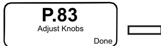
7. Turn the Volt Meter Calibration Adjust knob located under the volt meter on the user-interface until it matches the reference volt meter.
