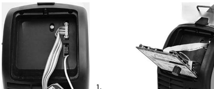
1. Fasten the cable connectors of the function panel to the power source (2 pieces).
